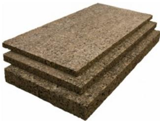
Cork insulation is made from the outer bark of evergreen oak trees grown in the Mediterranean. The bark is ground up into granules, which are then exposed to superheated steam. The granules are shaped into sheets and bound together by suberin, a natural binder. .
