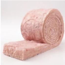
Fiberglass insulation is created when natural sand and recycled glass are fused together at a temperature of 2,640F. Individual fibers are created by forcing molten hot glass through a minuscule opening which creates a thin, small fiber, much in the same way that cotton candy is made. Resins and other chemicals are then added to make it heat resistant and to cement the fibers together.
