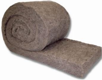
Wool insulation is made from sheep wool fibers. The wool used to manufacture insulation is the material discarded as waste by other industries due to color or grade. Some companies bind wool with 5%-15% recycled polyester adhesive which helps batts hold their shape. One can find wool insulation in the form of batts or rope (used primarily in log homes).
