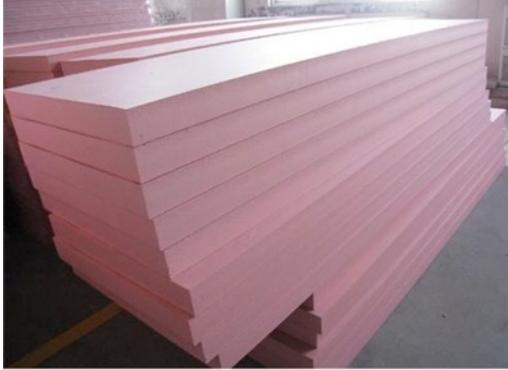
through a rectangular die, and then cut into sheets once cooled. XPS is midrange in cost and R-value when compared to the other rigid foams out there. It comes un-faced or with the option of different plastic facings. You can get XPS in low-density and high density options. The high density options are used in foundations, roofs, and other applications.
