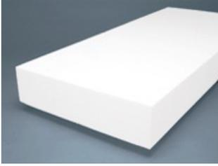
**PROS:** Expanded polystyrene is the least-expensive rigid foam insulation option. EPS typically uses pentane rather than high global warming potential CFCs as a blowing agent. Lightweight, resists moisture, doesn't need specialty tools for installation, can be installed by do it yourselfer and is highly resistant to air infiltration (from wind, etc...). EPS uses 1/7 of petroleum based products when compared to XPS.
