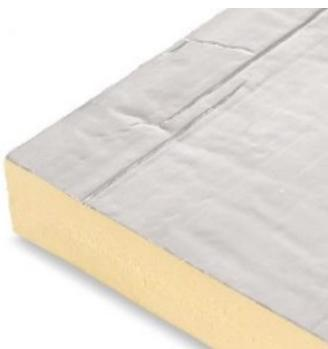
Polyisocyanurate (polyiso for short) foam is high density and made from a closed cell structure rigid insulation board. All ISO panels are faced. Foil-faced ISO panels are impermeable and create an exterior vapor barrier. Therefore, they shouldn't be used with interior vapor barriers.
